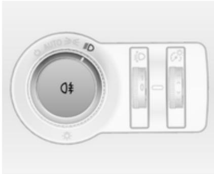
Wird durch Drücken von
