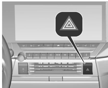
Wird durch Drücken von
