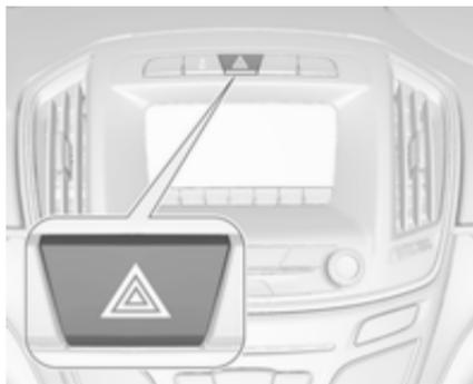
Wird durch Drücken von
